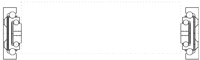
Standard application: Drawer extension telescopic rails vertical.
