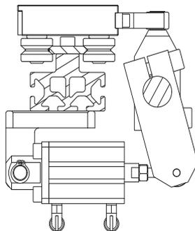
One cylinder is used to activate several positioning cam follower. Normal maximum length for a single unit up to 2000 mm.
