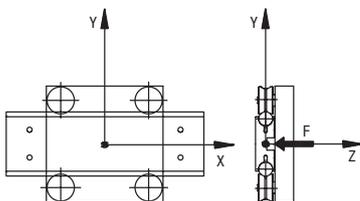
The external load F acts in the z-axis direction: P<sub>z</sub> = F = 2000
