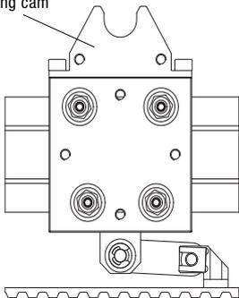
Positioning system is driven by pneumatic cylinder. Consider there is a space below the system and beside the carriages required for the air cylinder.
