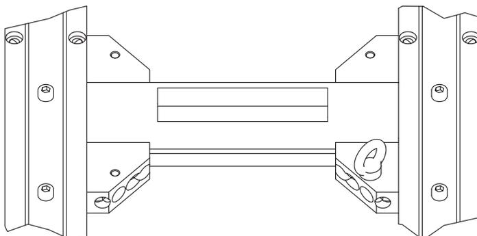
In case of long or heavy modules these can be provided with transversal supports (Option 14).
